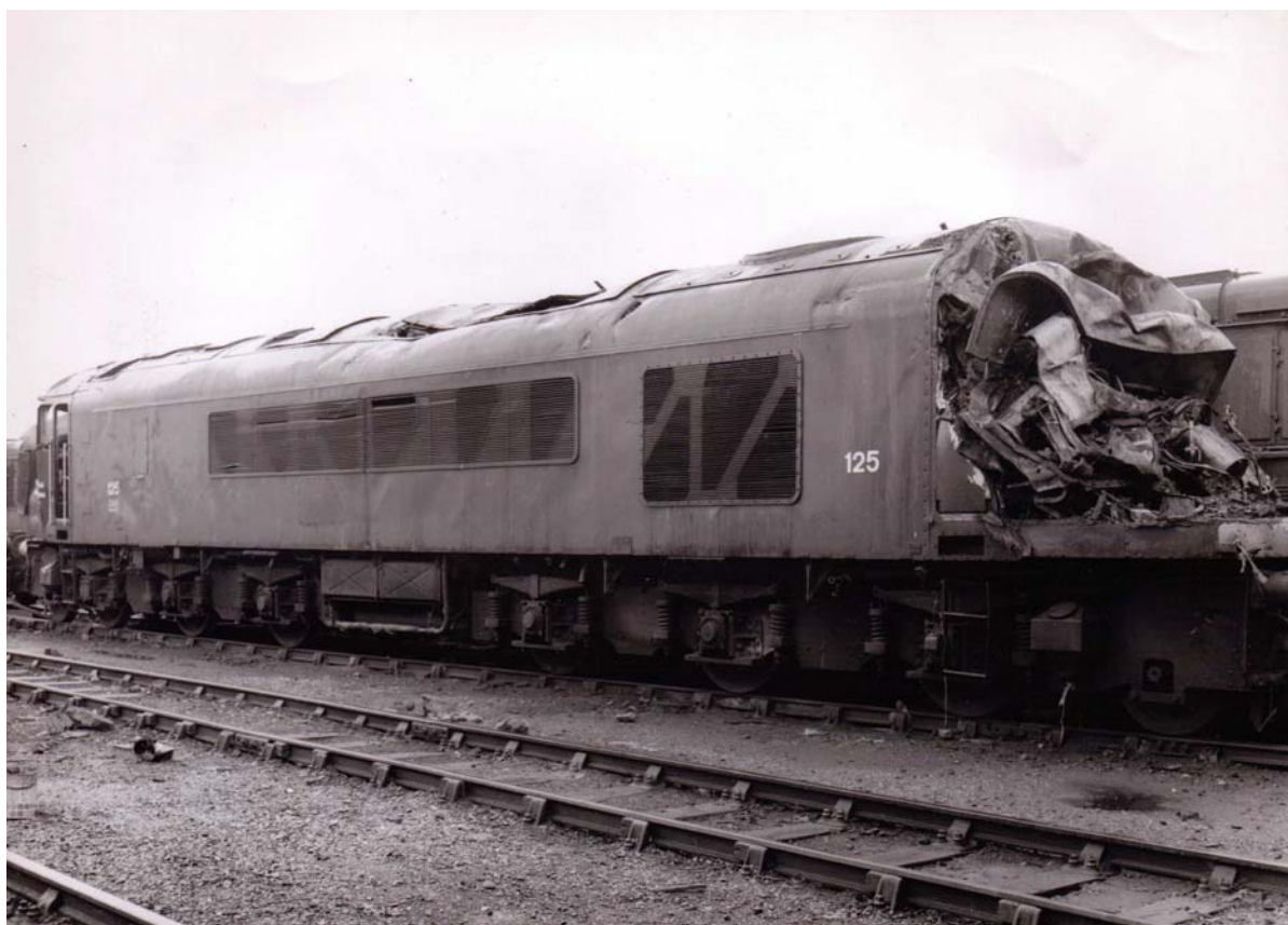
125 stored at Derby Works in early 1975, showing the severely damaged rear cab.
