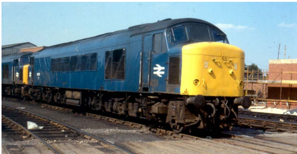
45071 shows off its new front end, with Class 20 style lights in 1976.
