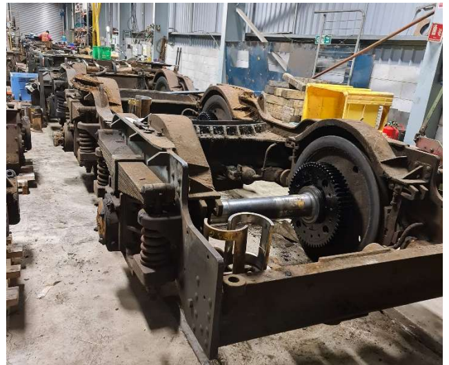
Bogies under overhaul at Barrow Hill on 26/01/21
