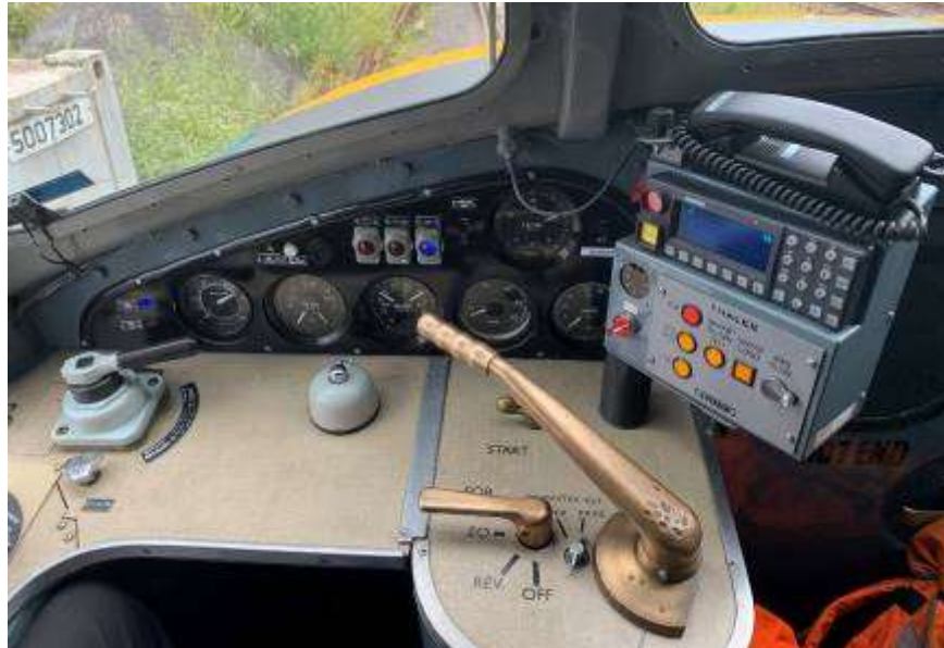
45118's No.1 end cab drivers desk, showing the sympathetic modifications to incorporate the TPWS and GSMR equipment to the right of the power handle.
