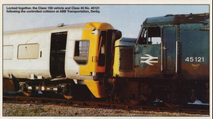
A CLASS 158 vehicle coupled to a ballasted flat wagon, to simulate a two-car Class 158 unit, has been rammed into 'Peak' locomotive No. 45121 at ABB Transportation's Litchurch Lane Works in Derby.
