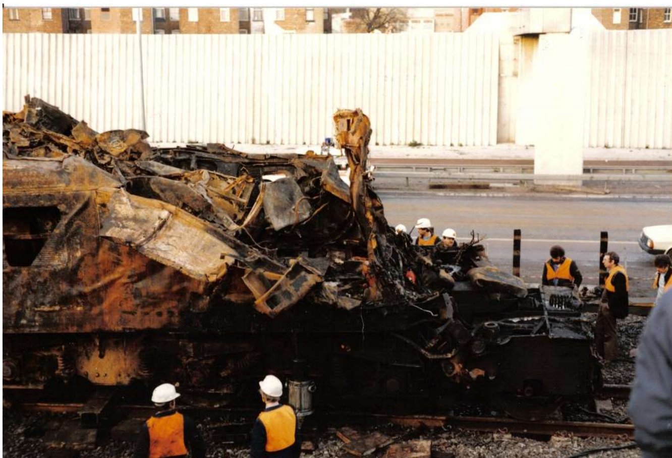
Above: The completely destroyed leading No.2 end of 45147 seen during recovery operations. Photo: F J Bullock
