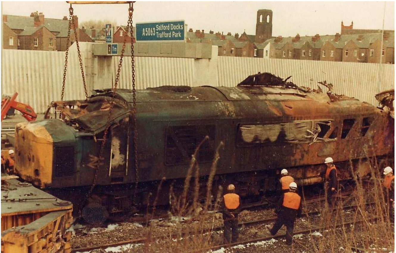
Above: Recovery of 45147 taking place on Wednesday 5 th December. This photo shows the extensive fire damaged and the crushed rear No.1 end cab. Photo: F J Bullock
