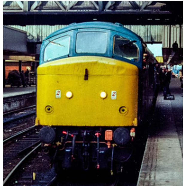
45147 seen at Leicester in April 1983, with the additional lamp bracket now fitted at No.2 end to match the other end.
