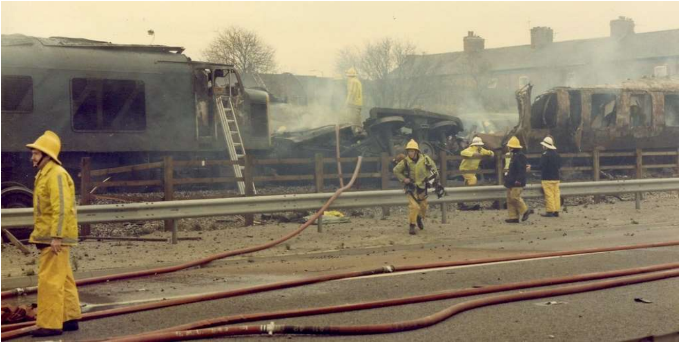
Above: The rear cab of 45147 and the remains of the leading Mk1 coach No. E3603. The front half of the coach body has been completely destroyed and the whole coach gutted by fire. A bogie from a tank wagon can be seen lying against it.
