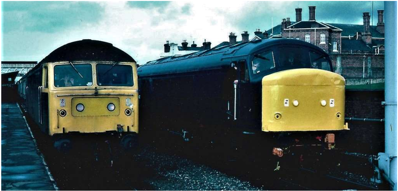
45147 can be seen at Shrewsbury on 14 th January 1983 during its first test run from Crewe Works. Note that the leading No.2 end does not have the upper lamp bracket fitted. Photo: Steven Clements.
