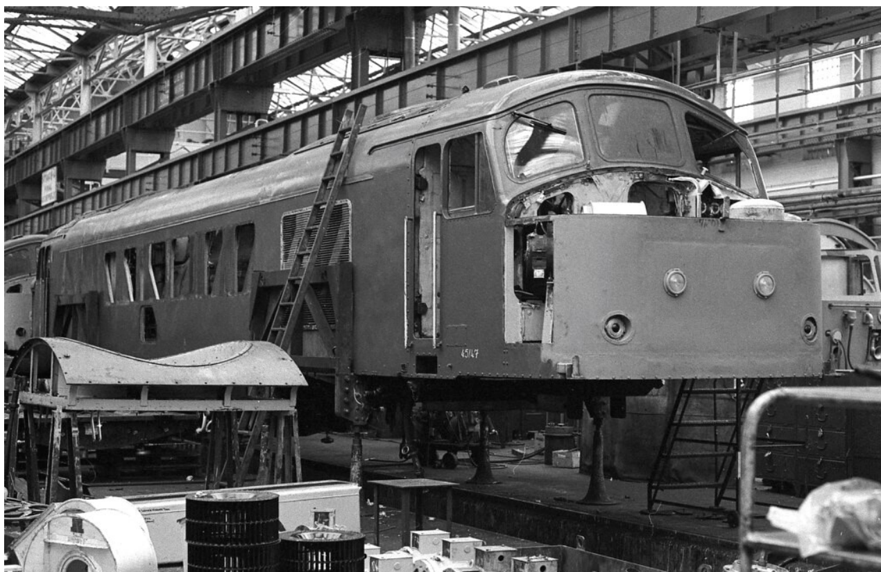
In this photo taken on 17 th October 1982, reconstruction of the No.1 end nose is nearly complete. However, the small handrails by the tail lights have not been replaced and the centre lamp bracket is still in place at the top. Photo: Kevin Connolly
