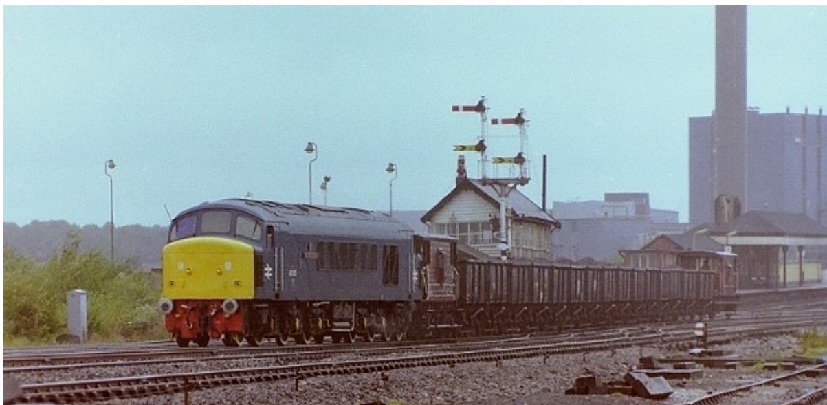
Just two days after its special working to Tees Dock, 45055 hauls a less glamorous ballast train past Miles Platting. Note the OLE warning signs mounted higher up the nose end than usual. Photo: Roger Varley 22/08/82.
