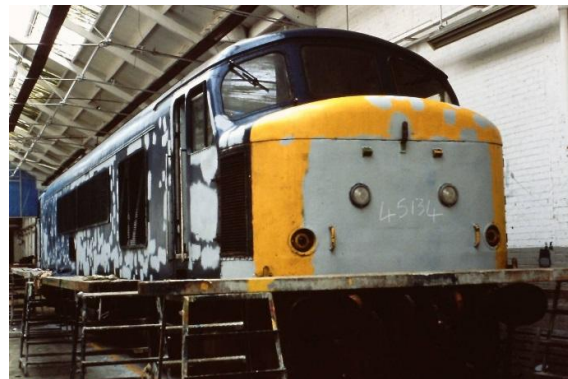
45134 in Crewe Works, 26/02/83, showing upper lamp bracket and headboard clips left in place after removal of headcode boxes.
