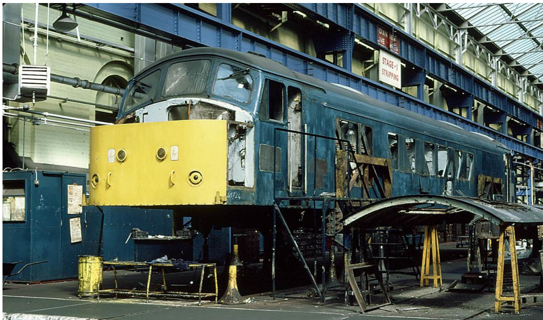
45124 undergoing a Heavy General Overhaul at Crewe Works in May 1982. Photo: Martin Addison
