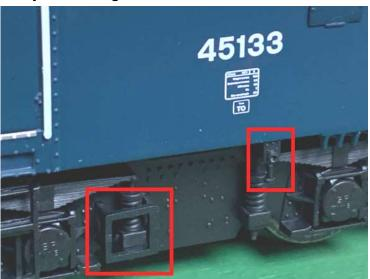
two items on the model which should not be present on a 45/1 (indicated on the picture left) – the first is the boiler water drain/filler cock on both sides at the No.2 end of the bodyshell. The second the are additional steps on the bogies, where
